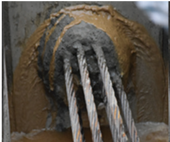
(a) Corrosion of strands due to flushing the PT ducts with water before grouting
